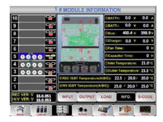
Fig. 52. Information menu of the module or power modules. Information sub-menu.
