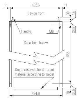
Dimensions for fixing the 6-slot sub-rack through its base
