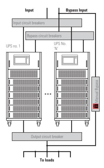
Fig. 35. Example of parallel system, with independent static bypass line and manual bypass board.
