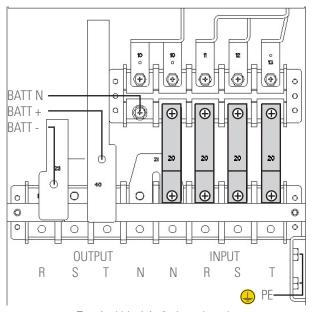
Terminal block in 8-slot sub-rack.
