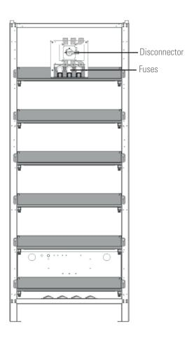
Fig. 8. Rear view of battery cabinets.
