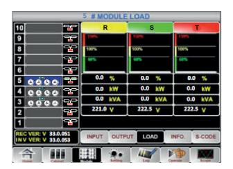
Fig. 56. Information menu for the power module or modules.
