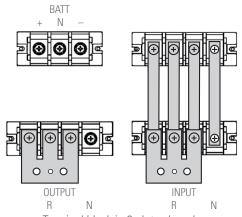
Terminal block in 6-slot sub-rack.
