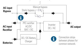
Fig. 20. Flowchart in Bypass mode.
