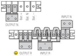
Terminal block in 2-slot and 4-slot sub-rack.
