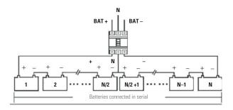
Fig. 32. Typical connection of battery set.
