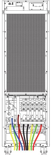
Fig. 31. Cable entry on 6 and 8-slot sub-racks.
