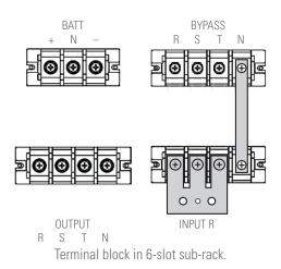
Fig. 16. Single-phase/three-phase configuration and separate networks.
