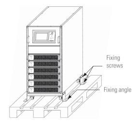
Fig. 26. Device unpacked on a pallet by way of example.
