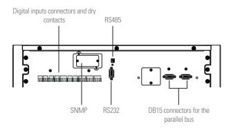
Fig. 38. Communication connections in 6 slot models.
