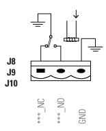
Fig. 44. Terminal block J8 and J9, and J10 relay interface.
