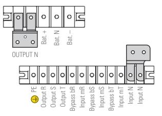
Terminal block in 2-slot and 4-slot sub-rack.
