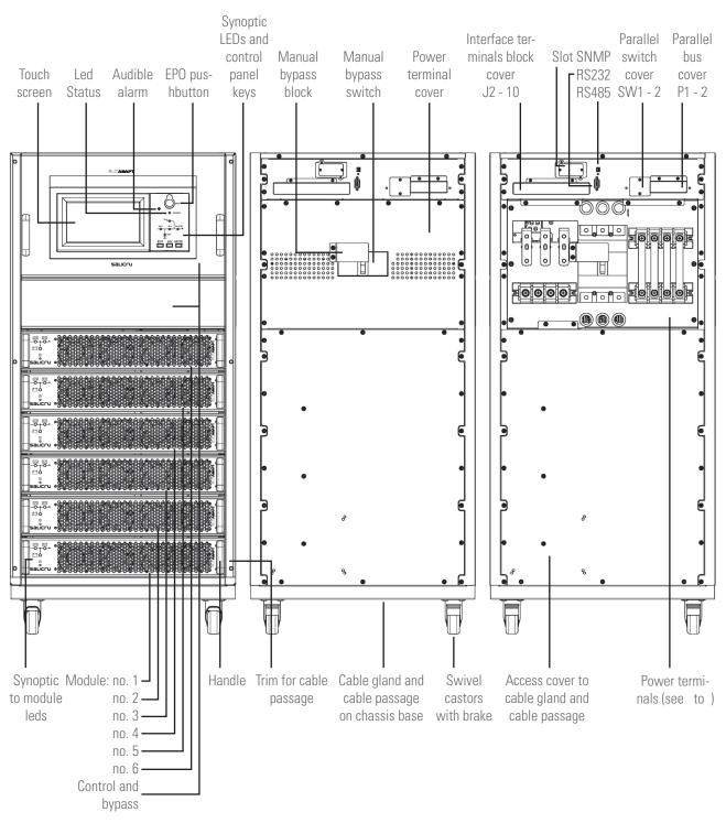
The figure on the right shows the sub-rack with the terminal cover removed.
