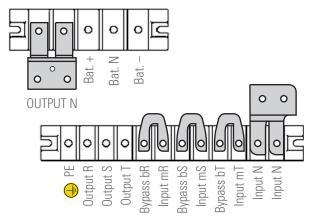
Terminal block in 2-slot and 4-slot sub-rack.
