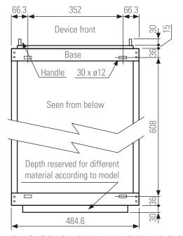
Dimensions for fixing 2 and 4-slot sub-racks through the bases
