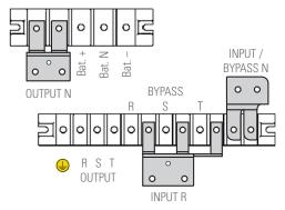
Terminal block in 2-slot and 4-slot sub-rack.
