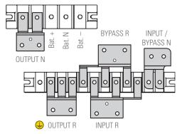
Terminal block in 2-slot and 4-slot sub-rack.
