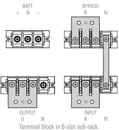
Fig. 14. Single-phase/single-phase configuration and separate networks.
