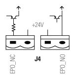
Fig. 40. Terminal block J4 for connection with external EPO.
