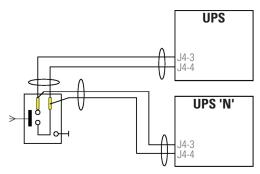
Parallel sub-racks connection with normally open contact -NO- in EPO.
