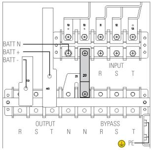
Terminal block in 8-slot sub-rack.
